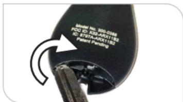
2. Place the key fob on a flat surface with the buttons facing down. Insert the tip of the emergency key or a flat head screwdriver into the area where the emergency key was located and twist to pop open the shell.
